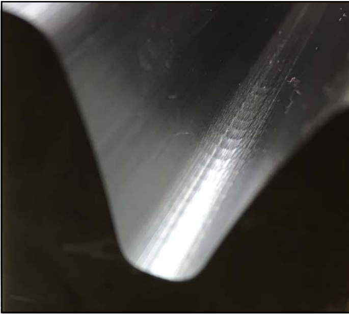
Figure 6 Chatter on gear tooth.
