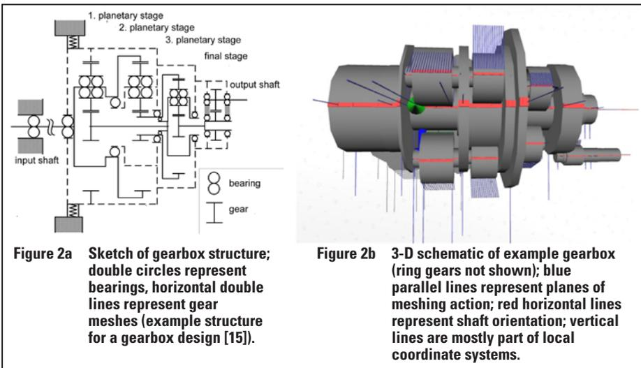
Figure 2a Sketch of gearbox structure; double circles represent bearings, horizontal double lines represent gear meshes (example structure for a gearbox design [15]).
