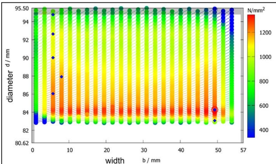
**Figure 9** Color-coded pressure distribution over area of tooth contact (same data as in Fig. 4). The local contact pressure is shown over the tooth flank; lines of contact are not indicated in this figure. Point A on the path of contact is located in the root area of the tooth flank; that range shows the highest pressure values.
