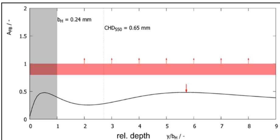
**Figure 10** Relative stress under tooth flank at evaluated point at about 88mm pinion diameter (Eq. 10) (see Fig. 9 for indication of the point by a blue square). The black line represents the risk of tooth flank fracture. The red area between values of 0.8 and 1.0 on the left axis specifies the critical range.
