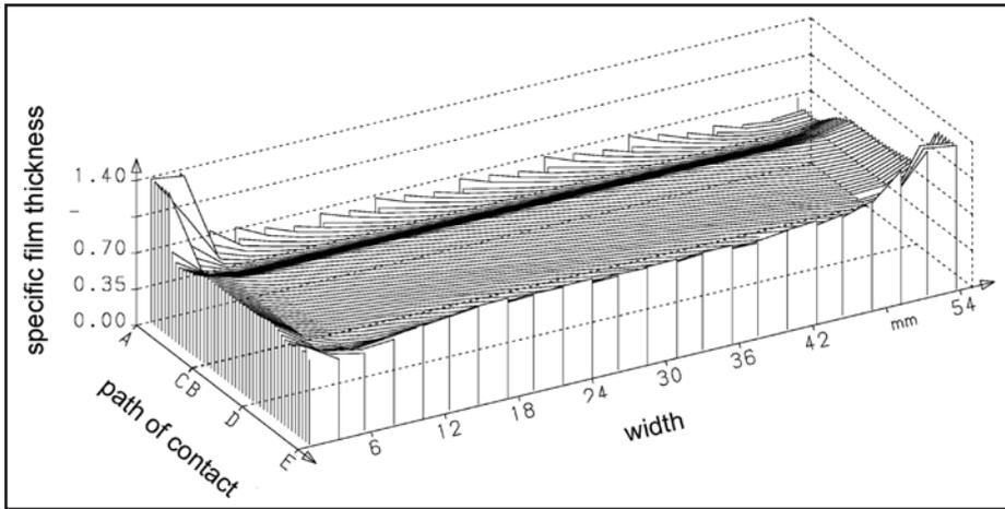
**Figure 8** Specific lubrication film thickness over the contact area. Every line represents a line of contact on the tooth flank and shows the resulting local specific lubrication film thickness (Eq.9).
