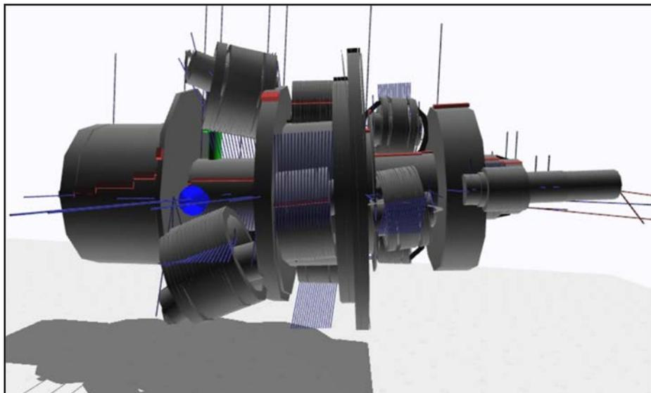
Figure 3 Scaled deformation of example gearbox under load.
