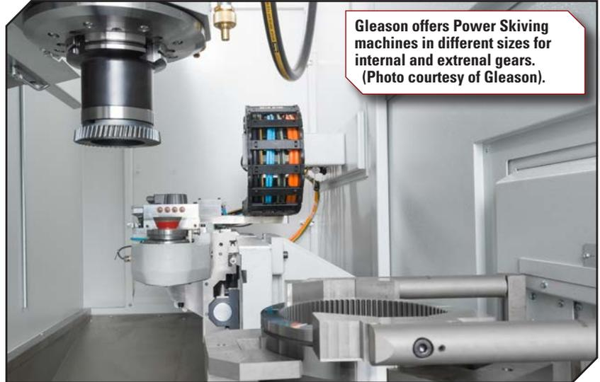
**Gleason offers Power Skiving machines in different sizes for internal and external gears. (Photo courtesy of Gleason).**
