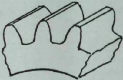
Fig. 4 – Spur Gear Tooth – Zero Helicoid
