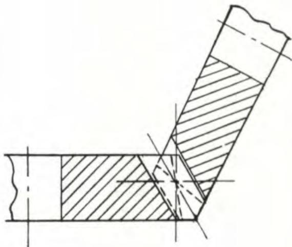
Fig. 23—Line of Contact — Non-parallel Axes
