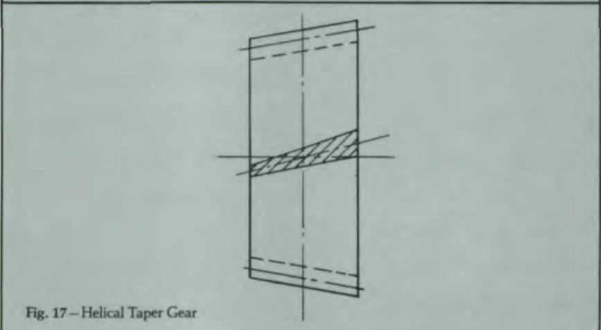
Fig. 17 – Helical Taper Gear
