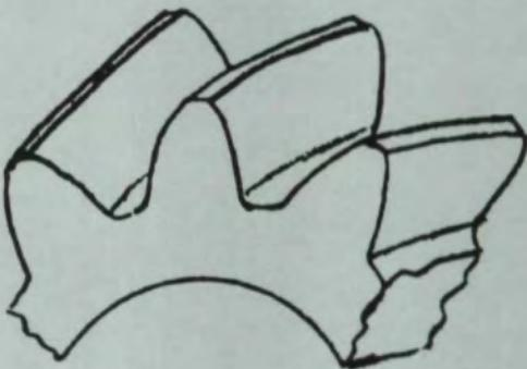
Fig. 5 – Helical Gear Tooth – Simple Helicoid
