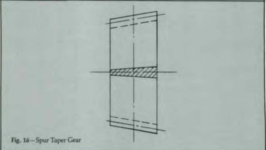
Fig. 16 – Spur Taper Gear
