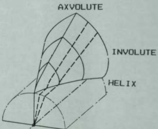
Fig. 6 – Spur Taper Gear Tooth – Complex Helicoid
