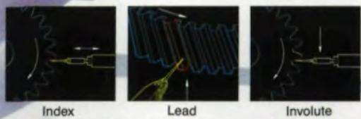
Process control can be implemented by analyzing data collected in gear testing. We offer SPC software to evaluate x-bar, R, histogram, and tooth surface topological studies.
