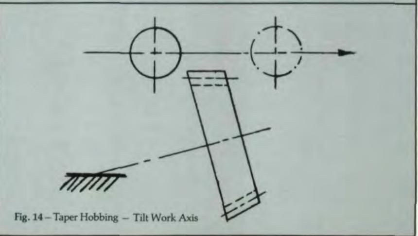
Fig. 14 – Taper Hobbing – Tilt Work Axis
