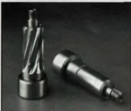
Dry hobbing produces Ford steering pinions in 48% less time, at 44% less cost and improved gear quality.
