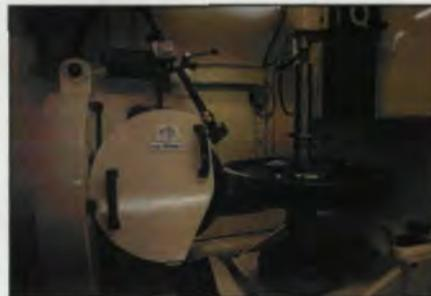
Fig. 2 – Cooper Turbocompressor gear being ground with 5° bevel.
